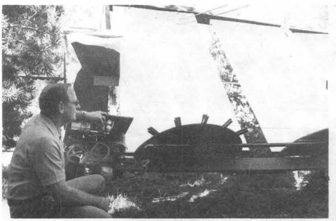
MANUAL OVERRIDE permits Clay Mavis (8451) to put his usually automatic heliostat through its sun-following paces. System supplies all hot water,
